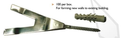
Galvanised Screwtie for inner leaf Galvanised to BSEN10111 1998 Stainless Steel Screwtie for outer leaf 304 Austenitic St / Steel to BSEN 10088-2/05 1.4301.
